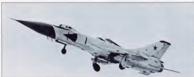
The first prototype Su-15 was rebuilt for STOL research. It had a modified wing and three additional engines; one was in the forward bay, with two in tandem to the rear. It was first flown in 1966.
